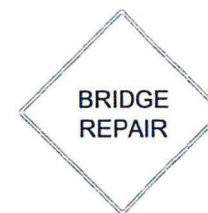
W21-9 BRIDGE REPAIR SIGN
