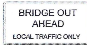
R11 BRIDGE OUT SIGN
