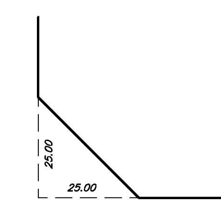
CHAMFERED CORNER DETAIL (NOT TO SCALE)
