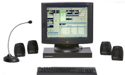
MCC 7500 Operator Position Components
